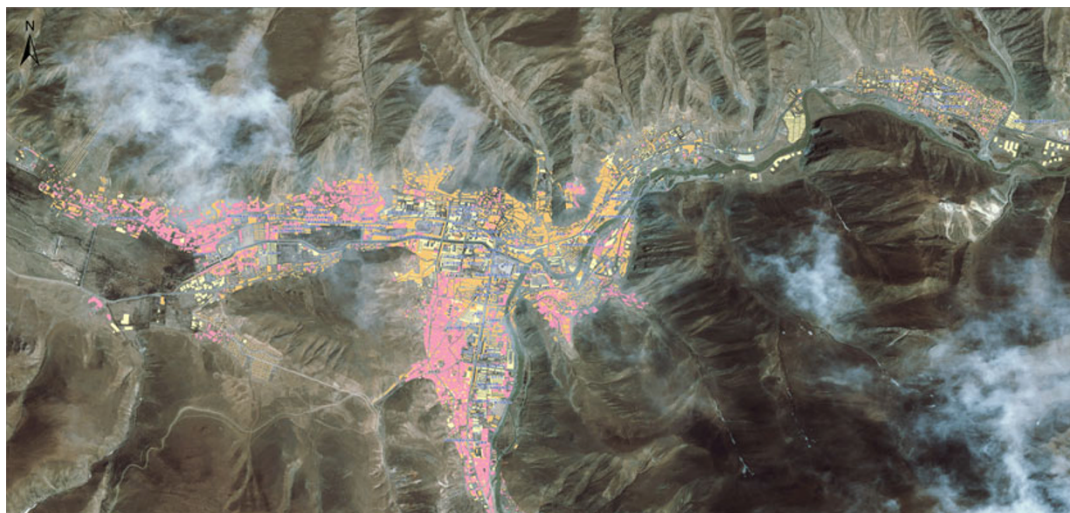
Figure 2. Remote-sensing assessment of collapsed and damaged houses in Jiegu Town (Pink identifies completely destroyed buildings, orange reflects severely damaged buildings, and yellow indicates slightly damaged buildings. The scale is 1:4000)
