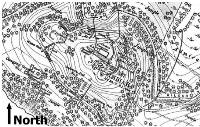
Plan for Imbiah Battery showing the infantry redoubt and the position finding cells and posts.
