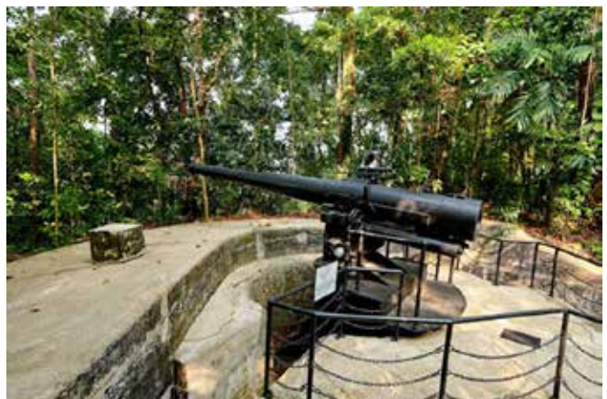
The 6 in QF battery at Fort Passeir Panjang. In 2002, an original 6 in barrel was mated with a replica central pivot mounting.
